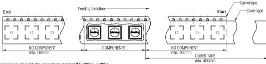
Packaging is referred to the international standard IEC 60286 -3:2007 Projection 165° -180° Würth Elektronik eiSos GmbH & Co. KG EMC & Inductive Solutions SSt JRS 6.3 2014-09-11 Max-Eyth-Str. 1 2014-04-01 SSt SSt 74638 Waldenburg Germany Pull-of force 2013-04-08 SSt COt Tel. +49 (0) 79 42 945 - 0 12 mm 0,1 N - 1,0 N www.we-online.com ME Tape width 6.0 2009-01-15 16 mm | 0,1 N - 1,3 N eiSos@we-online.com
