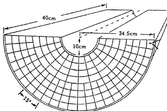
**Figure 1.** A SAT calorimeter halfbarrel. Each halfbarrel is subdivided into 144 readout elements.
