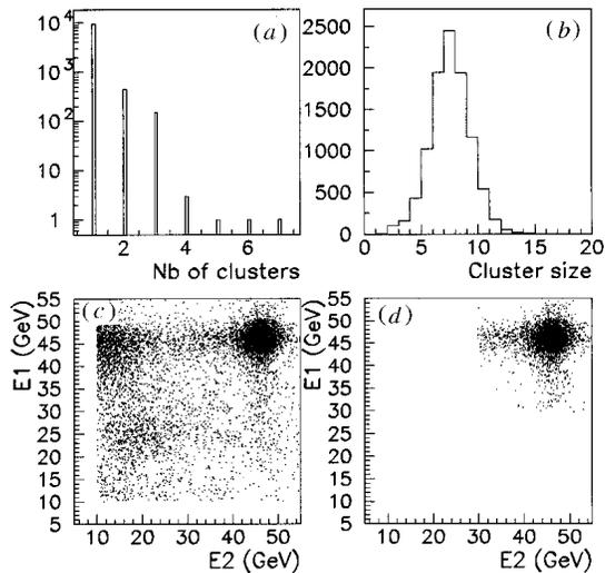
**Figure 3.** (a): Distribution of number of clusters per calorimeter. The data are observed to be largely dominated by one cluster per calorimeter (note the logarithmic scale). (b): Distribution of cluster size. (c): Energy in calorimeter 1 versus energy in calorimeter 2. No new cuts applied. Radiative tails and effects arising from a masking technique applied (see [5]) are clearly visible. (d): As in (c), but after the application of Bhabha event selection cuts (see the text).
