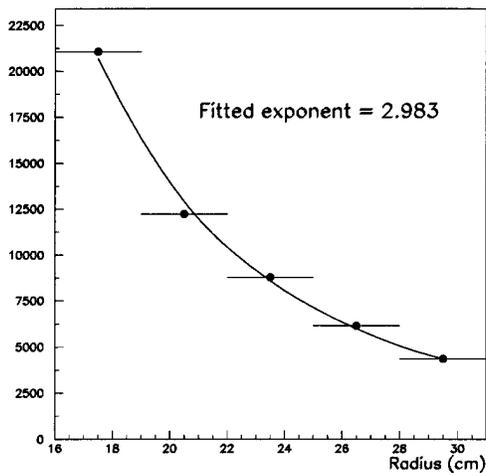
**Figure 4.** The radial distribution of Bhabha event energy clusters. A radial dependence  $f(R) = \text{constant} \times R^{-x}$  is fitted to the data. A value of  $x = 2.983$  is found, consistent with the theoretical prediction of  $x = 3$ .
