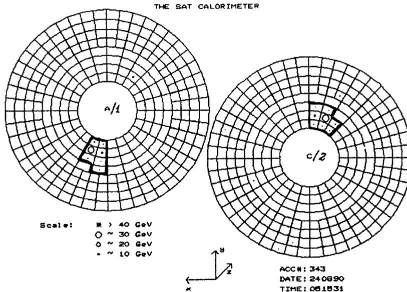
**Figure 2.** Energy depositions in the two calorimeters for a Bhabha event. The size of the rings which are drawn inside the hit elements is proportional to the deposited energy. Elements inside the borders drawn with a thick line are combined to clusters.
