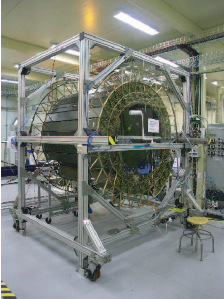
Figure C.6: The TRT detector, Barrel section, with two rings of modules installed and tested.
