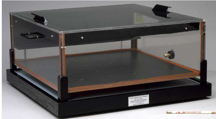
Figure 13.1: Cloud chamber [190] used at several exhibitions and outreach booths. The cooling dry ice is placed inside the black frame under the metal chamber floor. The cloth-covered brim of the chamber plexiglass box is moistured with alcohol and the alcohol vapor sinks to the bottom as it is being cooled. Incident particles leave “condense trails” very much like the familiar jet trails in the sky.
