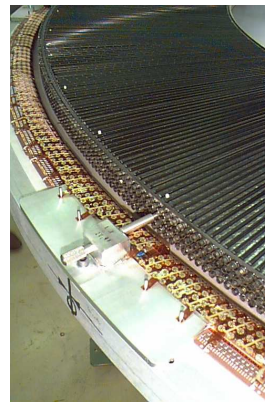
Figure 2.9: The TRT endcap with radially oriented straws (From ATLAS webpages).
