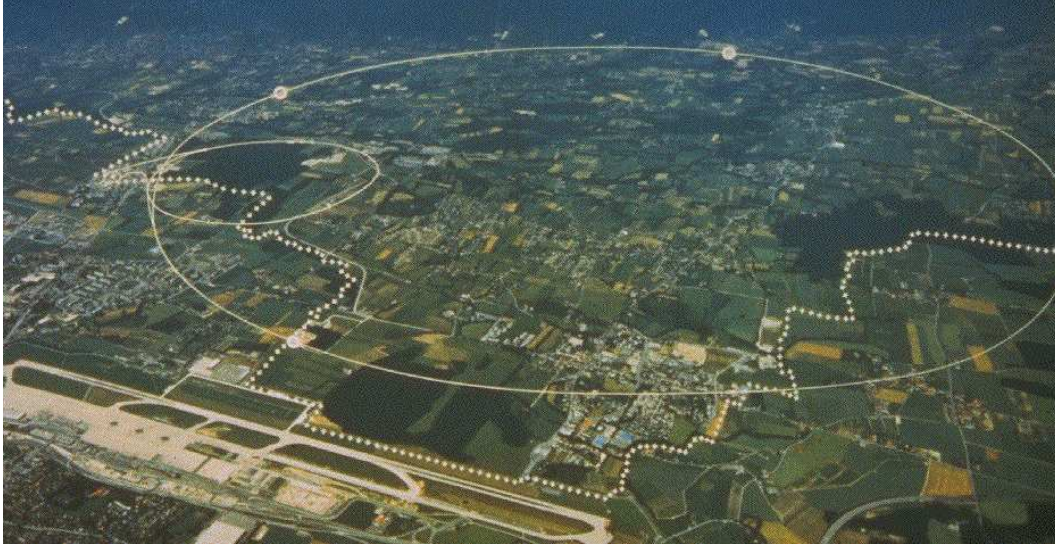
Figure 1.1: CERN is located near the point where the small and the large circle, indicating the SPS and LEP rings, coincides. The dotted line is the border between France and Switzerland, Geneva airport is seen near the bottom. The large dots on the LEP ring represents detectors, the dot closest to the airport indicates the position of DELPHI.
