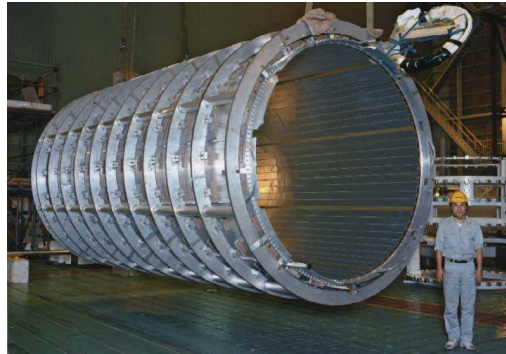
Figure 2.8: The solenoid magnet of the ATLAS detector.
