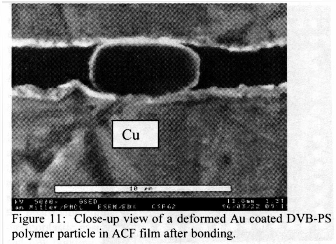
Figure 11: Close-up view of a deformed Au coated DVB-PS polymer particle in ACF film after bonding.
