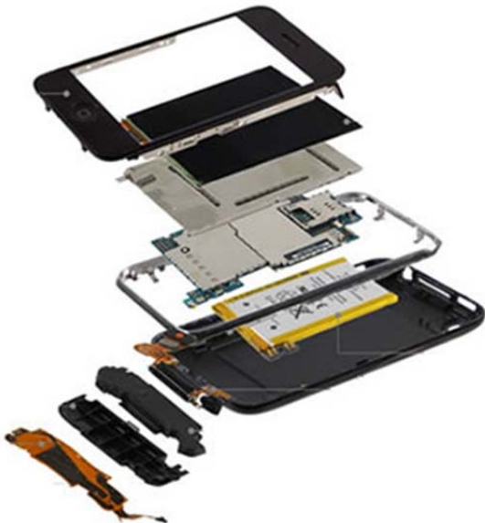
Fig 1: Sammenstilling av/Assembly of iPhone 3G S. Fra/From http://www.techspot.com/news/35215-isuppli-apples-iphone-3g-s-costs-179-to-make.html
