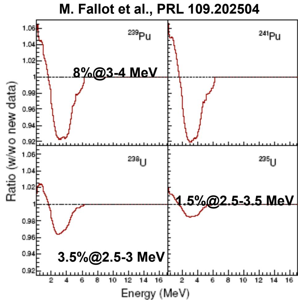
Ratio between 2 antineutrino spectra built with and without the  $^{102,104,105,106,107}\text{Tc}$ ,  $^{105}\text{Mo}$ ,  $^{101}\text{Nb}$  TAS data
