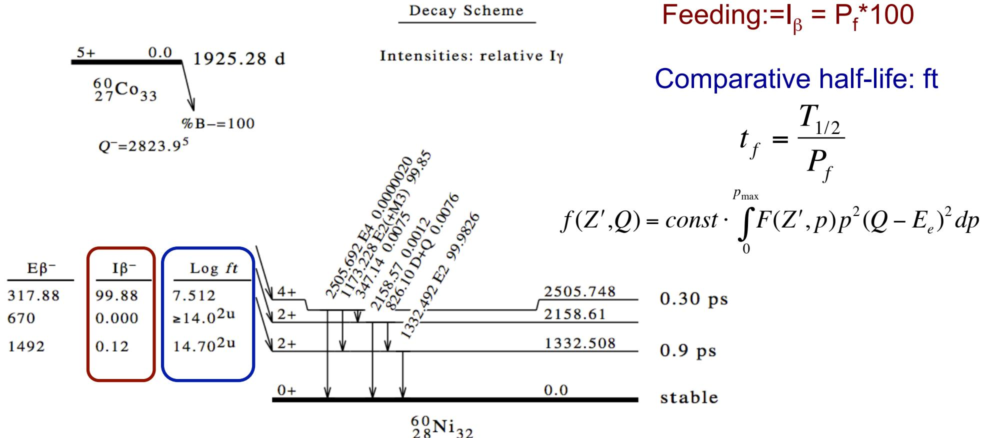
$$ft_f = \text{const}' \frac{1}{|M_{if}|^2} = \text{const}' \frac{1}{B_{i \rightarrow f}}$$
