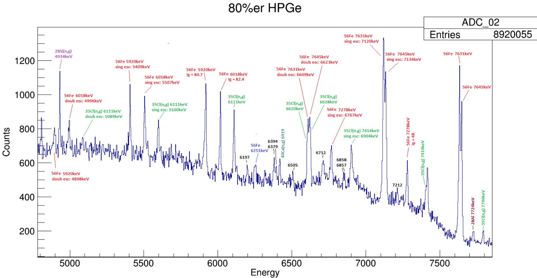
$^{56}\text{Fe}(n_{\text{th}},\gamma)$  is used for energy and efficiency calibration
