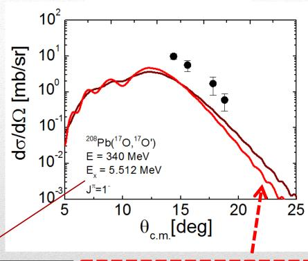
To understand the measured E1 cross sections, we have to perform DWBA calculations with a different type of nuclear form factor
