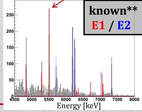
The Coulomb excitation cross section based on the B(E1) $\uparrow$  values known from  $(\gamma,\gamma)^{**}$  have been calculated
