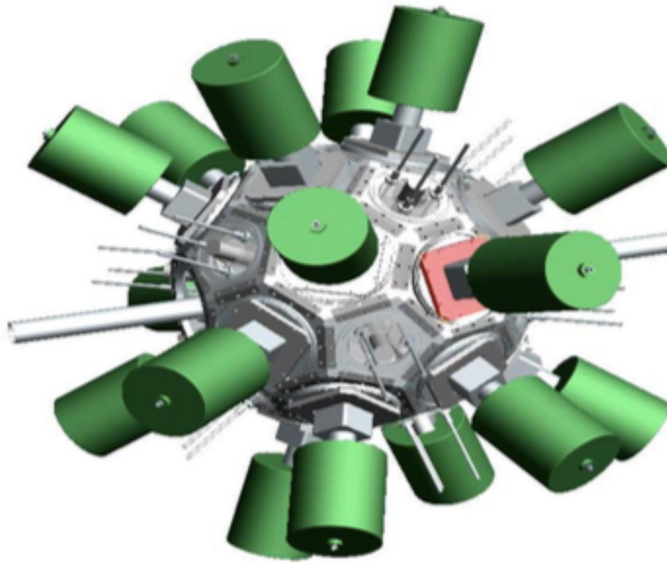
This unique experimental setup would pioneer a new generation of studies where the  $\gamma$ -decay probability is too low to be investigated with the current arrays located worldwide.
